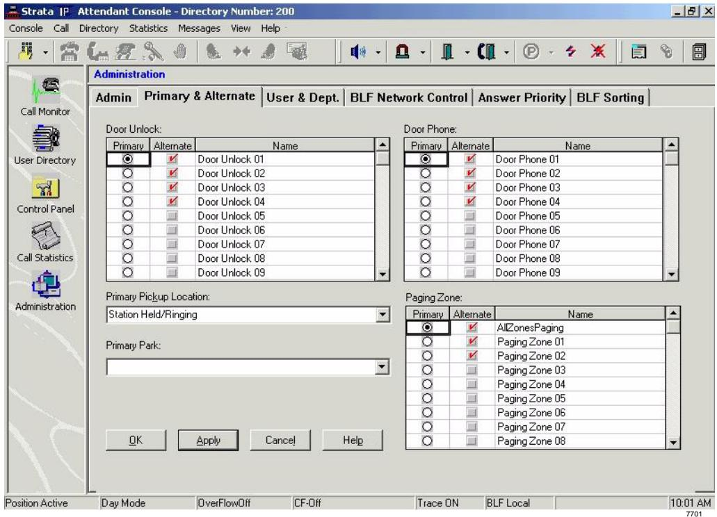
The number of doors and paging zones must match the number assigned in Strata CIX IP programming.
